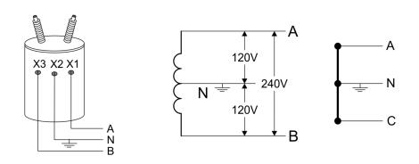
This single phase service is the most common for residential customers. It is also used for small commercial customers. A single center tapped transformer provides two hot lines and a neutral.
