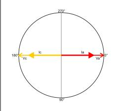
The meter phasors and the distribution phasors are identical.
