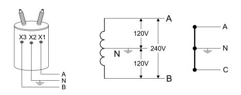
This single phase service is the most common for residential customers. It is also used for small commercial customers. A single center tapped transformer provides two hot lines and a neutral.
