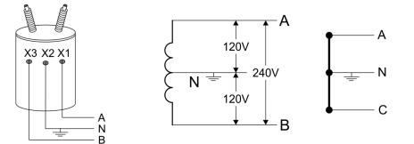
This single phase service is the most common for residential customers. It is also used for small commercial customers. A single center tapped transformer provides two hot lines 180 degrees out of phase and a neutral.
